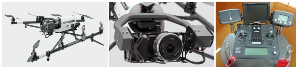
Fig. 4. UAV (Falcon 8) and facilities used for aerial photography
