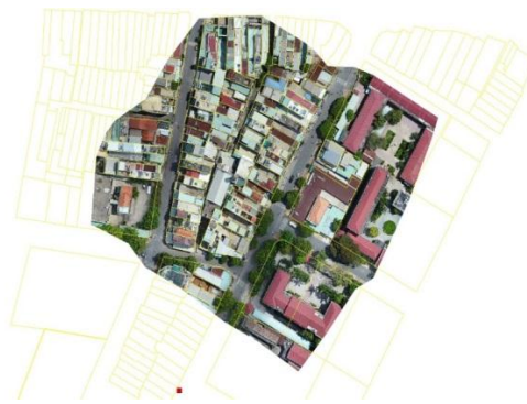
Fig. 6. Illustration on overlay ortho images with the parcel boundaries for updating the cadastral map
